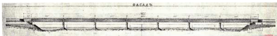
Fig. 1. Design of the bridge by Tadeusz Chrzanowski: 7 cross-bracing truss spans of 66.22 m + 2 plate structure spans of 15.24 m each.
